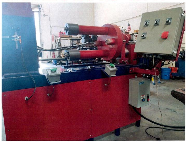
This is a very special unit that is designed to reduce heavy wall pipe that us use in the boiler production and repair industry. There are 4 stations on this particular unit. The capacity in terms of pipe diameters and wall thickness will determine the design of the structure and power supply. We build to our customers specifications. With this known, a product drawing of the product is needed
